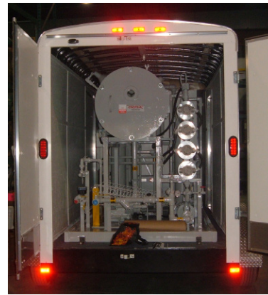
Enervac model E865A-1200 (1200 gph) oil purification processor shown in a dual axle cargo trailer.
