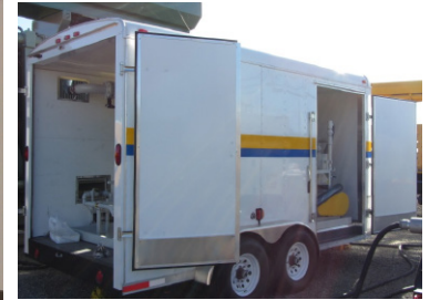
Enervac model E865A-1200 (1200 gph) oil purification processor shown in a dual axle cargo trailer.
